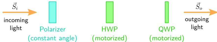
**Figure 2.3.:** Setup for the generation of arbitrary polarization states using a polarizer with a constant angle and a motorized HWP and QWP.
