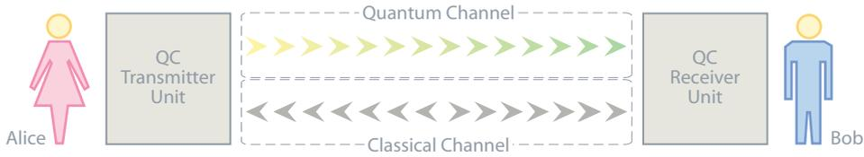
**Figure 3.1:** Alice can secretly communicate with Bob using an additional trusted quantum channel and a classical channel. The key-exchange procedure occurs through the quantum channel. Once the quantum transmission is over, they check whether the key is secure and, if so, they can use it to encrypt confidential data through the classical channel.
