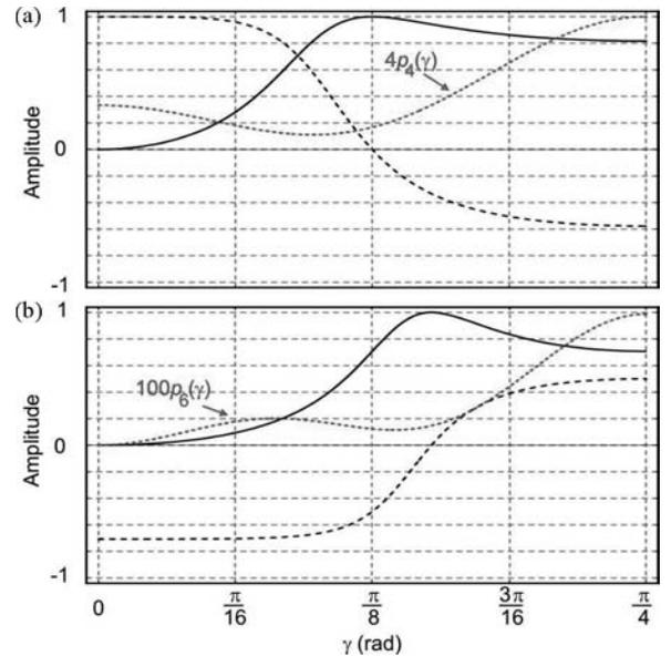
Fig. 2. Amplitudes. (a)  $a_4(\gamma)$  (solid) and  $b_4(\gamma)$  (dashed) for the family of states  $|\Psi_4(\gamma)\rangle$ . (b)  $a_6(\gamma)$  (solid) and  $b_6(\gamma)$  (dashed) for  $|\Psi_6(\gamma)\rangle$ . Further, (a)  $p_4(\gamma)$  and (b)  $p_6(\gamma)$  denote the probability of each state to be observed in the corresponding linear optical setup (dotted).
